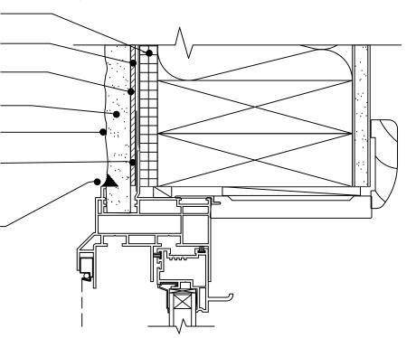
SCS 06\_01 WINDOW FIN INTERFACE WITH INTEGRAL EXTRUDED RECEIVER
