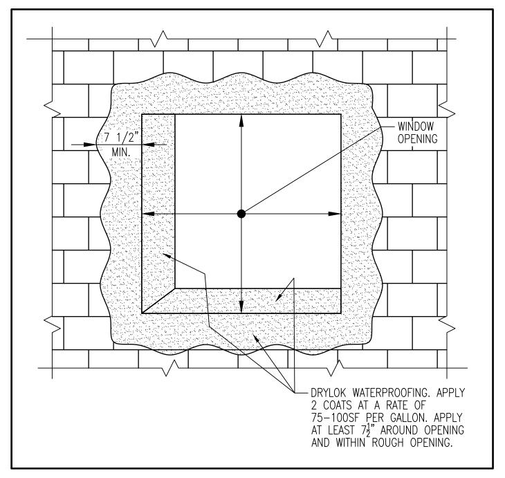
DRYLOK CONCRETE/MASONRY WATERPROOFER
